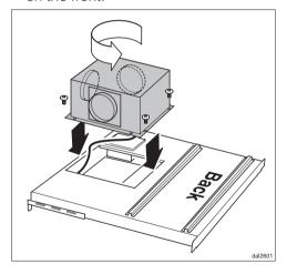
■ Mount the blower on the rear the same way as described for mounting on the front.
